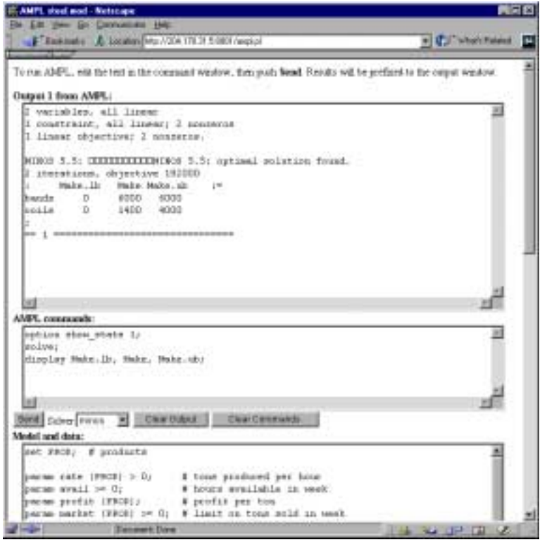
Figure 1: The “Try AMPL” server’s result screen includes an output window (at top) and a solver menu and other controls. The contents of the commands and model/data windows may be modified and resubmitted.
