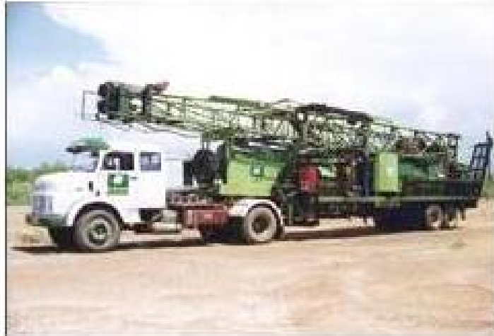
Fig. 2. Transportation of a workover rig
