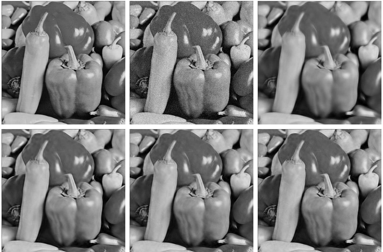
Figure 8: Denoising of Peppers . From left to right and top to bottom: original; noisy; iteration #1; iteration #2; iteration #3; final.
