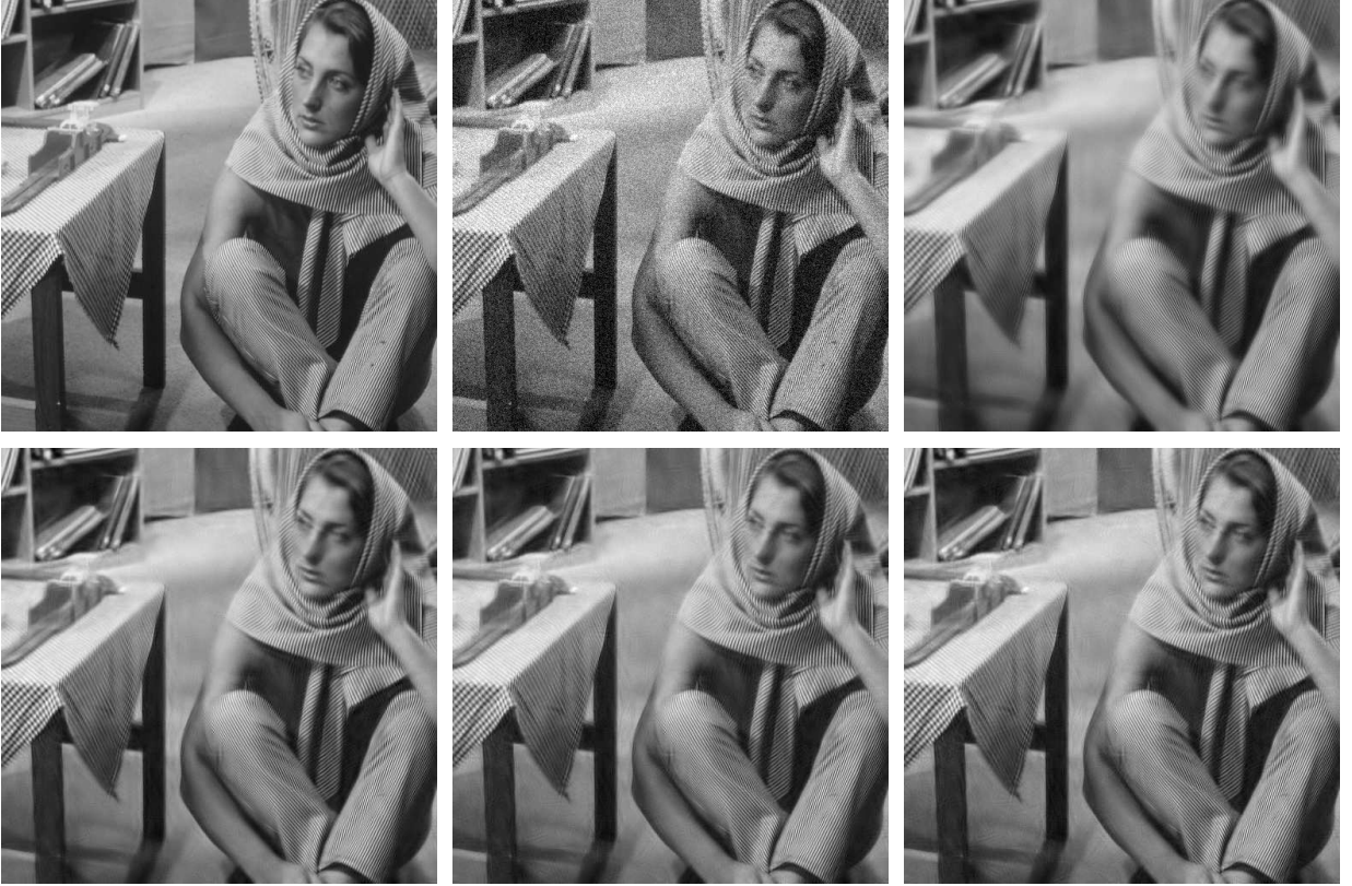
Figure 9: Denoising of Barbara . From left to right and top to bottom: original; noisy; iteration #1; iteration #2; iteration #3; final.
