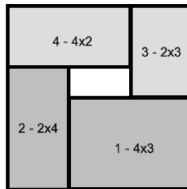
FIGURE 8. Example of an instance with a 6 \times 6 stock rectangle and single copies of 4 \times 3 , 2 \times 4 , 2 \times 3 , and 4 \times 2 rectangles to be packed. The optimal solution is shown in the figure. For this instance, the Bottom-Left (BL) placement heuristic cannot produce the optimal solution.
