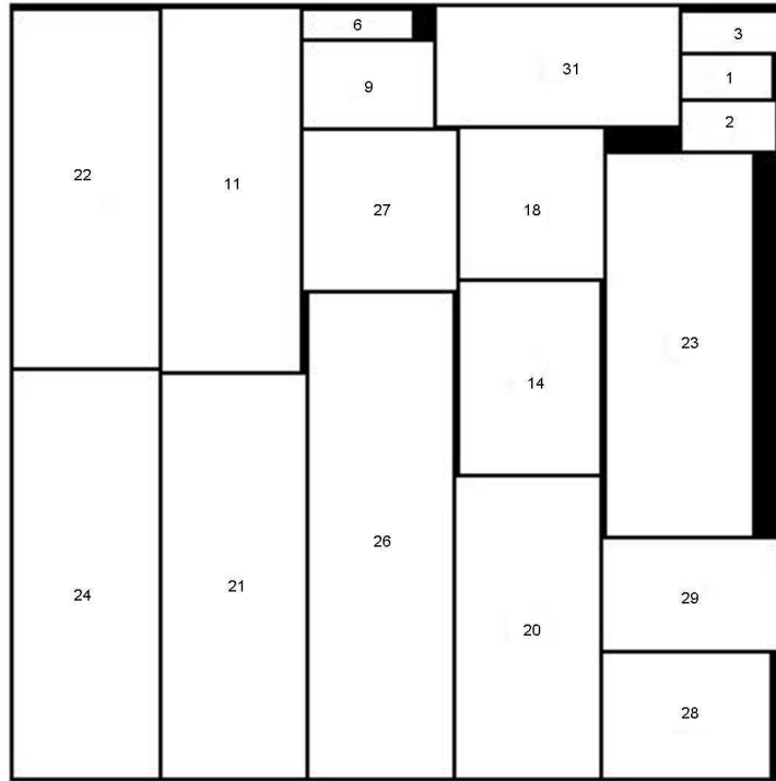
FIGURE 15. Best solution found by HH for problem instance gcut13 using RPS = \{24, 21, 26, 20, 28, 29, 22, 11, 27, 9, 6, 14, 18, 31, 23, 2, 1, 3, \dots\} and VPP = \{BL, BL, BL, BL, BL, BL, BL, LB, LB, LB, LB, LB, LB, LB, LB, BL, BL, BL, BL, BL, \dots\} . Total value of packing is 8,654,707, which is a new best known solution (BKS) for the problem instance. The previous BKS was 8,281,060 and was found by the genetic algorithm (GA) of Hadjiconstantinou and Iori (2006).
