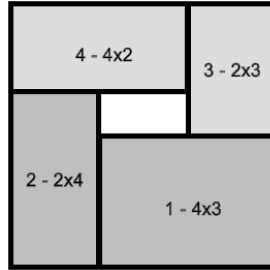
FIGURE 10. Optimal solution, for the problem in Figure 8, found by combining the Bottom-Left (BL) and the Left-Bottom (LB) placement procedures. First, rectangle 2 (of size 2 \times 4 ) is placed with BL. Then, rectangle 1 (of size 4 \times 3 ) is placed with BL. This is followed by rectangle 4 (of size 4 \times 2 ) which is placed with LB. Finally, rectangle 3 (of size 2 \times 3 ) is placed with BL.
