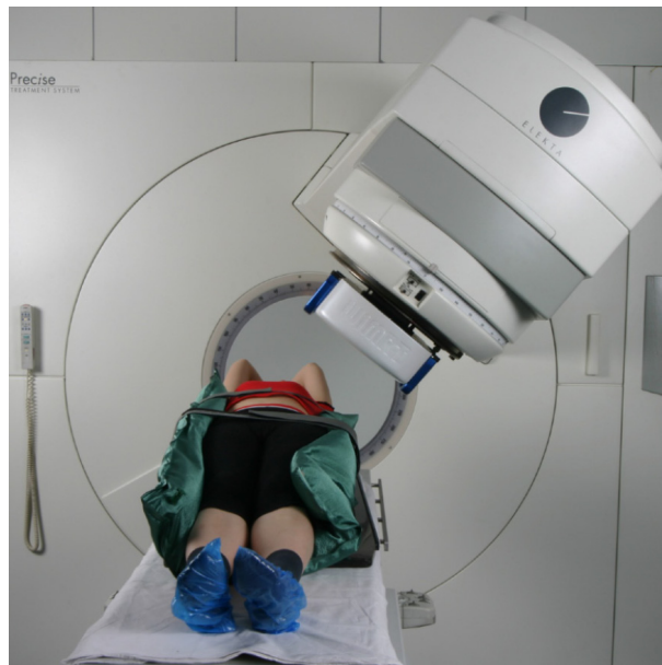
Figure 4-12: A typical oncology system used in IMRT. The radiation beam can be directed onto a patient from different angles, because the equipment can be rotated about an axis. Credits to: Rismed Oncology Systems, http://www.rismed.com/systems/tps/IMG_2685.JPG , April 15, 2007.
