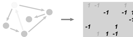
Figure 4: A node and all incoming arcs deleted by user presolving. Notice that two of the remaining arcs have no source.
