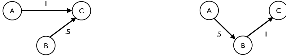
Figure 6: Monday load plan does not consolidate Figure 7: Tuesday-Friday load plan consolidates freight through BB terminal B .
