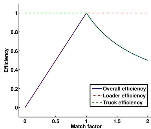
**Figure 6** The Match Factor (MF) is the ratio of loader productivity to truck productivity. A low MF ( $< 0.5$ ) suggests that the loader is not working at capacity, whereas a high MF ( $> 1$ ) suggests the truck fleet is smaller than necessary to maintain a productivity balance between truck and loader fleets.
