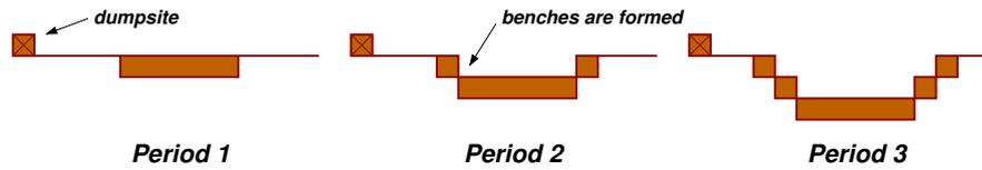
**Figure 1** A mining schedule is divided into planning periods. In each period, the mine planning decisions include which material will be excavated, and where the excavating equipment and stockpiles will be located. For a long-term schedule, these periods could be one year in length.
