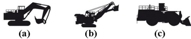
**Figure 2** Excavating equipment may include (a) hydraulic, (b) rope and (c) front-end loaders. Images from Immersive Technologies (2012)
