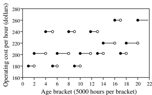
**Figure 4** This figure describes the discretized operating cost function over time. The rise in operating cost reflects the increased maintenance expense; large drops in the expense occur when a significant maintenance, such as overhaul, has taken place.
