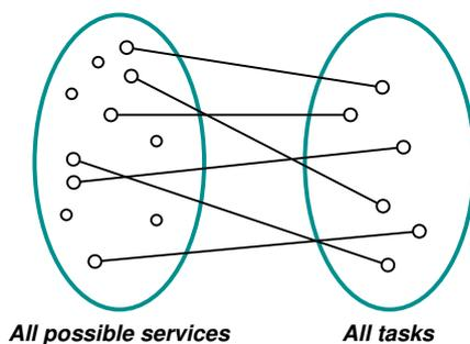
**Figure 5** The allocation and dispatching problems are concerned with matching services (e.g., provided by equipment) to tasks (e.g., moving ore).
