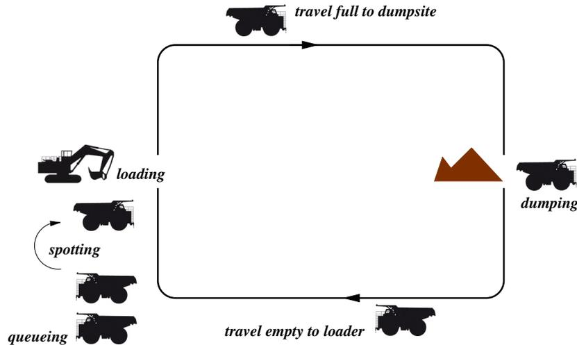
**Figure 3** The truck cycle time is measured from the time the truck is filled at the loader, travels full to the dumpsite, dumps the load, and travels empty to the loader to join a queue and positions itself for the next load (spotting). The truck cycle time includes queuing and waiting times at the dumpsite and loader. Images adapted from Immersive Technologies (2012)
