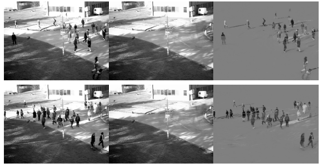
Fig. 2. Left: Original frames of a video (436 384 × 288-pixel frames). Middle and Right: recovered background (low-rank) and foreground (sparse) components.
