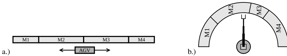
Figure 1: In a.) an AGV transports parts between the machines moving in both directions along a straight line. In b.) a material-handling industrial robot carries parts between the machines.
