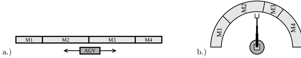
Figure 9.1: In a.) an AGV transports parts between the machines moving in both directions in a straight line. In b.) a material-handling industrial robot carries parts between the machines.
