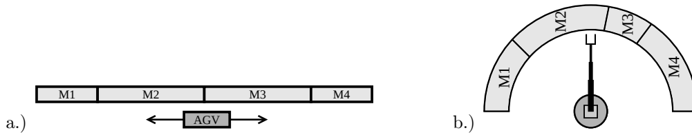
Figure 10.1: In a.) an AGV transports parts between the machines moving in both directions along a straight line. In b.) a material-handling industrial robot carries parts between the machines.
