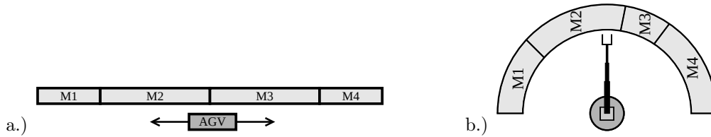
Figure 2.1: In a.) an AGV transports parts between the machines moving in both directions along a straight line. In b.) a material-handling industrial robot carries parts between the machines.
