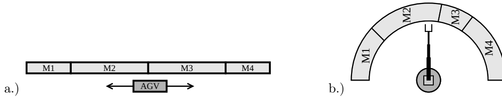
Figure 12.1: In a.) an AGV transports parts between the machines moving in both directions along a straight line. In b.) a material-handling industrial robot carries parts between the machines.
