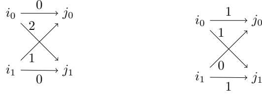
(a) Initial flow in which we want to increase the flow between i_0 and j_0 . (b) Flow after increasing the flow between i_0 and j_0 by \bar{x} = 1 .
