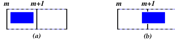
Figure 5 The two cases of equipment age landing between periods. For case (a), the equipment stays in the same age bracket for the entire period. In case (b), the equipment steps over into the next age bracket within the period.
