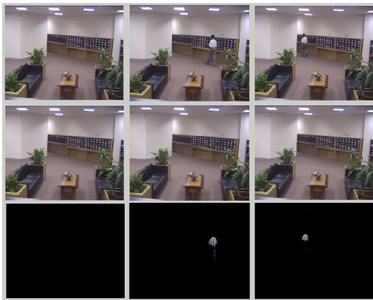
Figure 2: Robust Video Recovery. The first row are the 3 frames of the original video sequence. The second row are recovered background. The last row are recovered foreground.
