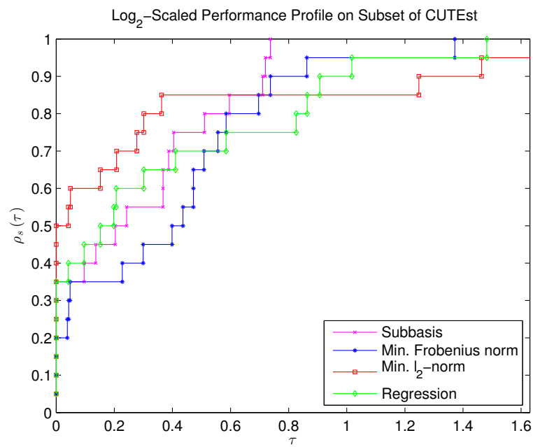
Figure 5.3: \text{Log}_2 -scaled performance profile of DEFT-FUNNEL with different approaches to build the models on a set of 20 linearly constrained problems from CUTEst.
