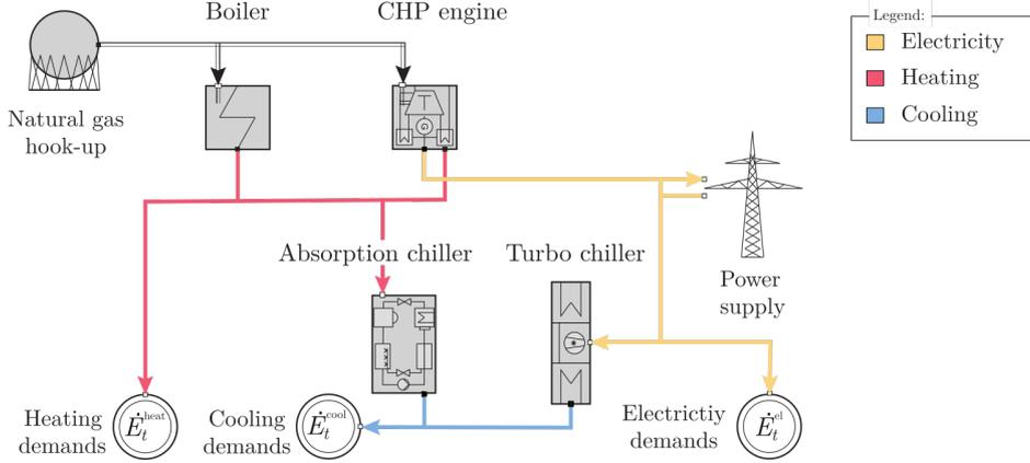
Fig. 1. Example of a decentralized energy supply system.
