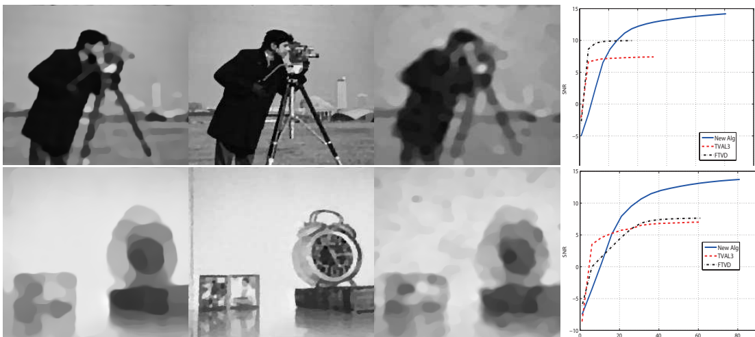
Figure 1: From left to right are the results of FTVD, New algorithm, TVAL3, and SNR history plot. First row: NR = 60%; second row: NR = 80%.
