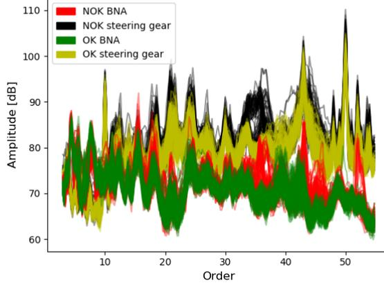
Figure 1: Overview of the connection between the BNA and the steering gear by means of the 300°/s averaged order spectrum plot for 70 OK and 70 NOK pairs. The 'NOK' BNA label refers to the case when the corresponding steering gear was faulty due to the BNA, even though the BNA had passed its own vibrational test.
