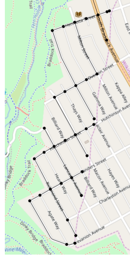
(b) The plowing graph is limited by an artificial district border on the right. The routing graph however expands beyond the border, thereby drastically reducing the number of U-turns needed if the streets would end at the district border.
