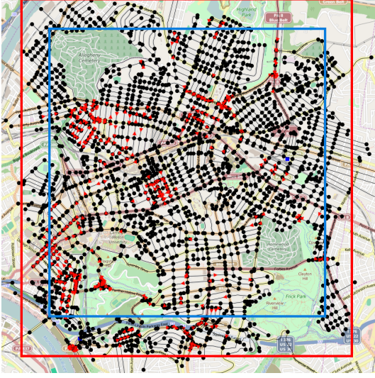
(a) The plowing graph, marked by the blue rectangle, is a subgraph of the routing graph, delineated by the larger red rectangle.
