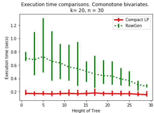
Figure 10 Execution times (in secs) of compact LP and row generation for various tree heights, n=30 , k=20
