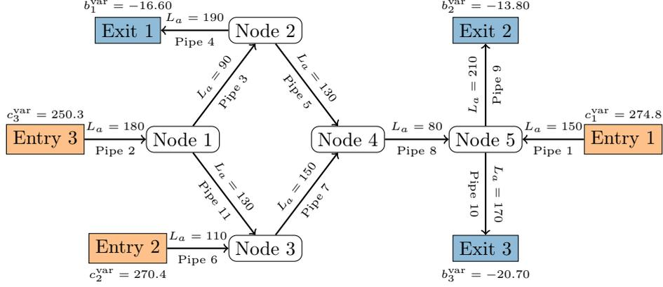
FIGURE 1. Gas network considered in the numerical study with variable costs  $c_i^{\text{var}}$  (in EUR/(1000 Nm<sup>3</sup>/h)) of entries, slopes  $b_i$  (in EUR/(1000 Nm<sup>3</sup>/h)<sup>2</sup>) of exits, and length  $L_a$  (in km) of pipes.
