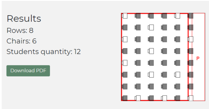
Fig. 9: Student distribution result, with the fixed chairs option selected. This example was generated in a 6m \times 8m room, with 8 rows of 6 chairs, measuring 0.5m \times 0.5m each, maximizing the number of students considering a 1.5m distance between them. We can see that, in this case, 12 students can be accommodated, as shown by the white chairs.
