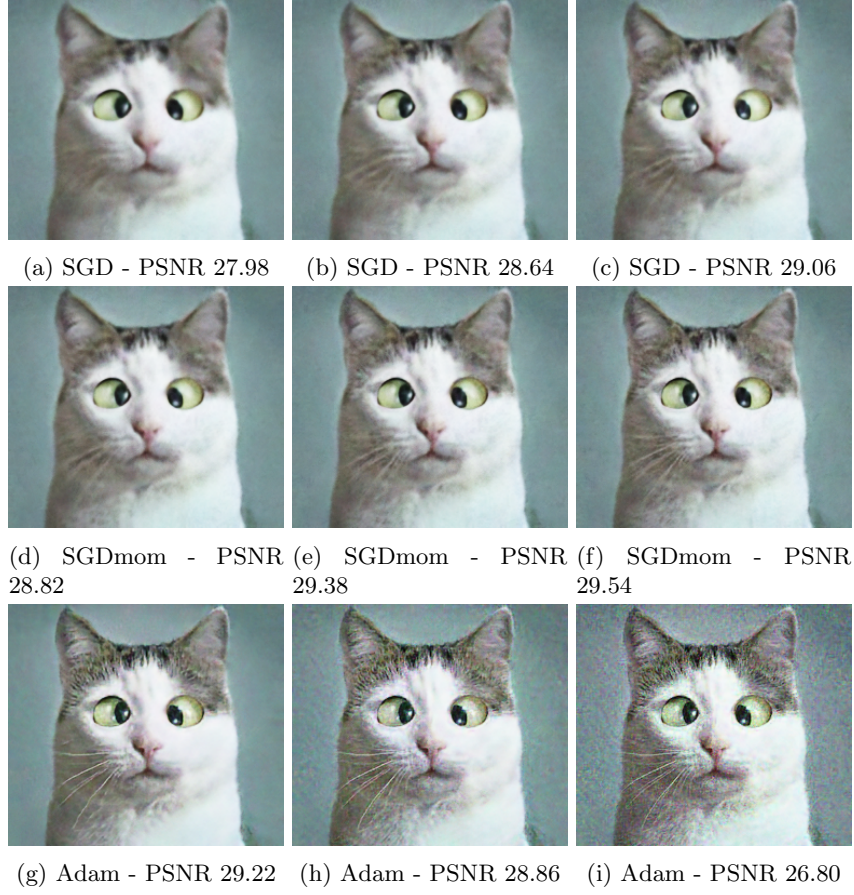
Figure 5: Images obtained at a fixed number of iterations, for different methods. First column iteration 2600, second 4000 and third 5400. First row SGD (LR=0.5), second row SGDmom (LR=0.1) and last row Adam (LR=0.01). In the caption the PSNR of each reconstruction
