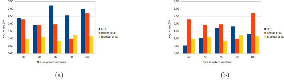
Figure 3: Average relative optimality gaps, depending on the number of vertices in the instances. Comparison of literature LP bounds with the LP bound of our formulation (Fig. 3a) and with root node bound of algorithm \mathcal{F} (Fig. 3b).
