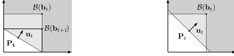
(a) Minimum-volume box containing the intersection. We maintain sets of low-complexity by computing the minimum-volume box \mathcal{B}(\mathbf{b}_{t+1}) containing the intersection of the initial box \mathcal{B}(\mathbf{b}_t) and the half-space \mathcal{H}_{<}(\mathbf{u}_t) obtained from Proposition 4.3 when the preconditioner \mathbf{P}_t fails to yield sufficient decrease. (b) Need sufficient backtracking. If the candidate preconditioner \mathbf{P}_t selected inside the initial box \mathcal{B}(\mathbf{b}_t) is not close enough to 0, there might not be a box smaller than \mathcal{B}(\mathbf{b}_t) that contains the intersection.
