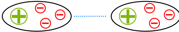
Fig. 2: London dispersion: the formation of instantaneous dipoles due to electron density fluctuation.
