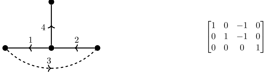
Figure 2. Digraph, spanning tree (plain edges) and network matrix. The arcs are numbered to match the column ordering
