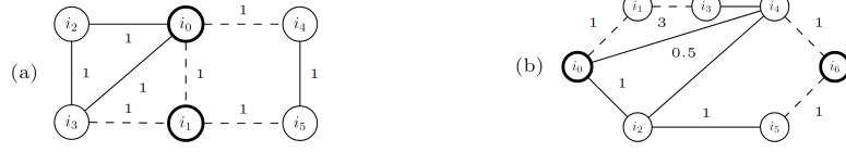
Fig. 3: Examples of situations where the reachability set should be refined: (a) In \mathcal{C}_{i_0 i_1}^N , \{[i_2, i_3], [i_3, i_3]\} are replaced by [i_0, i_3] , as \{(i_0, i_2), (i_0, i_3)\} \in \Omega^0 ; (b) In \mathcal{C}_{i_0 i_6}^N , [i_4, i_4] , [i_4, i_5] , and [i_2, i_4] are replaced by [i_0, i_4] , since \{(i_0, i_2), (i_0, i_4)\} \in \Omega^0 , and since [i_0, i_4] is connected in G^0 , [i_0, i_4] also replaces [i_1, i_4] .
