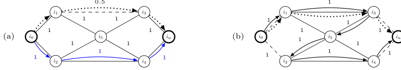
Fig. 2: Tightening SPP- and LPP-based angle difference bounds using path-based VIs: (a) Bus pair [i_0, i_n] is connected in G^0 and a potential path (dotted arrows) shorter than the SPP-based path exists; (b) Bus pair [i_0, i_n] is disconnected in G^0 and a potential path (dotted arrows) shorter than the LPP-based path exists.
