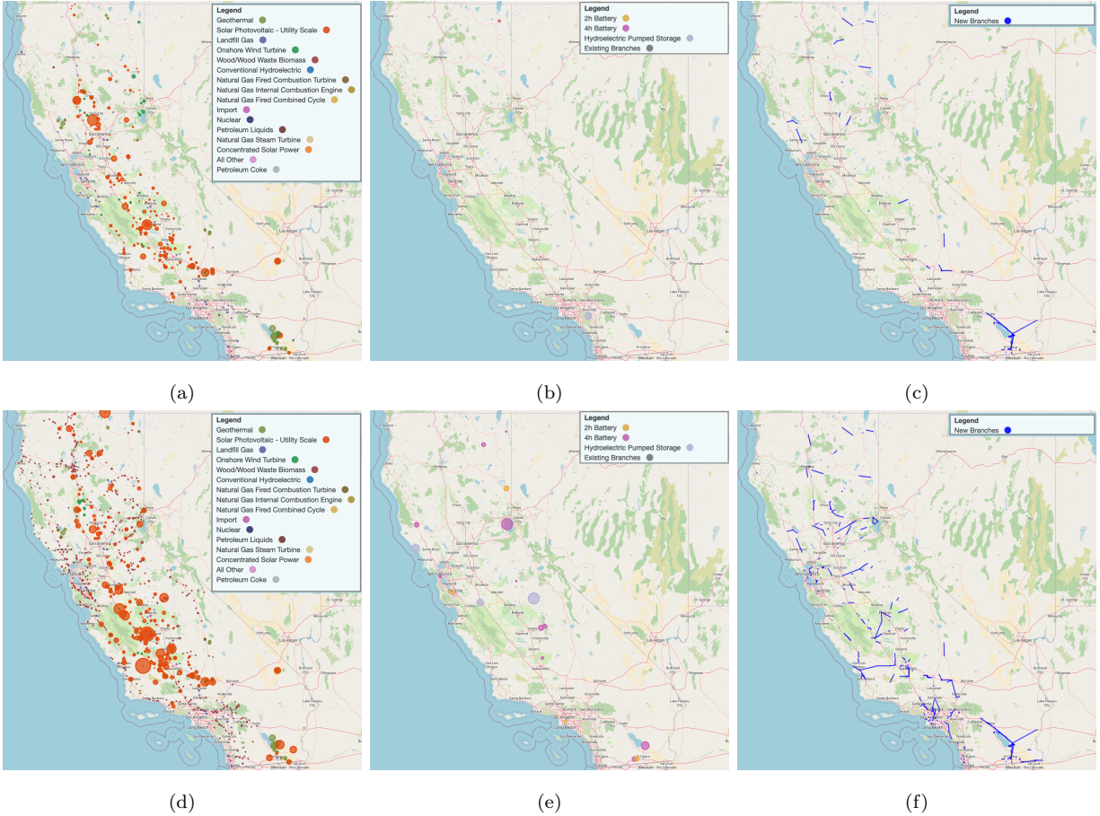
Figure 4: Comparison of new generator, storage, and transmission line locations for 2019 (a – c) and 2045 (d – f). The area of the circular markers is proportional to capacity.
