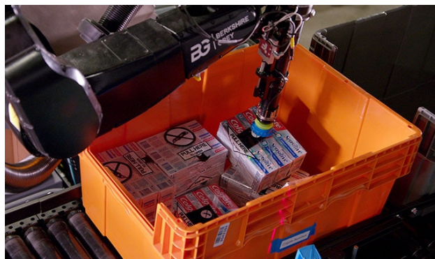
Figure 1: A robot arm picking an individual product from a case (Berkshire Grey 2022)
